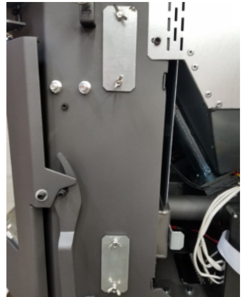
Figure 25: Exhaust Chamber Cover Plates. (Air Intake side)
