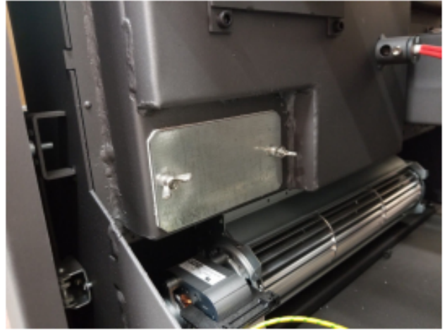
Figure 25: Exhaust Chamber Cover Plate. Air Intake side
